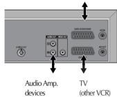
To copy to your player from another video machine, connect the two machines with a cable between their EURO AV (SCART) sockets and select as programme "AV 1/AV 2" or "F. AV" (front sockets) using the [AV], [PR+/-] or [  $\Diamond$  ] button.
